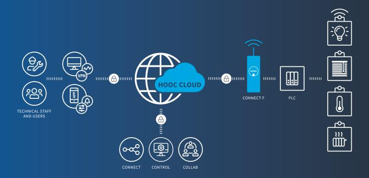
In practice (from left to right): The user (technical manager, operator, end customer, etc.) logs in via app or PC and receives access to the HOOC Cloud via a secure connection. From there, he can then access his PLC, HVAC systems or smart home applications thanks to the HOOC gateway. This high-quality VPN tunnel forms the basis for all other HOOC solutions in the Connect, Control and Collab area.
