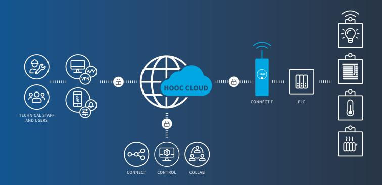
**In practice** (from left to right): The user (technical manager, operator, end customer, etc.) logs in via app or PC and receives access to the HOOC Cloud via a secure connection. From there, he can then access his PLC, HVAC systems or smart home applications thanks to the HOOC gateway. This high-quality VPN tunnel forms the basis for all other HOOC solutions in the Connect, Control and Collab area.
